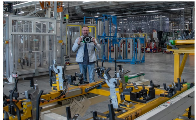
Figure 2. After signalling, the skid is simply photographed from different directions with the hand-held C1 Camera.
