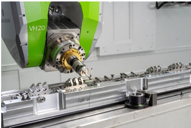
Figure 5. In-process measurement of the component is performed directly in the clamping to avoid measurement deviations due to spring back or warping.
