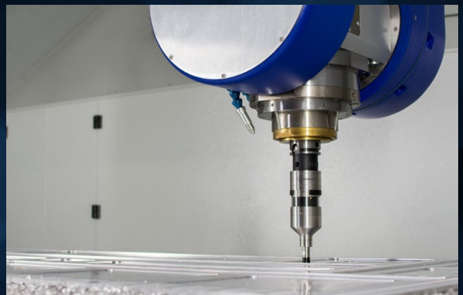
Figure 2. Automated wall thickness measurements on the machine tool with ultrasonic probes replace time-consuming manual measurements with external devices, without the need to move heavy and large parts to dedicated measurement spaces, ultimately resulting in significantly faster inspections and enhanced data capture.
