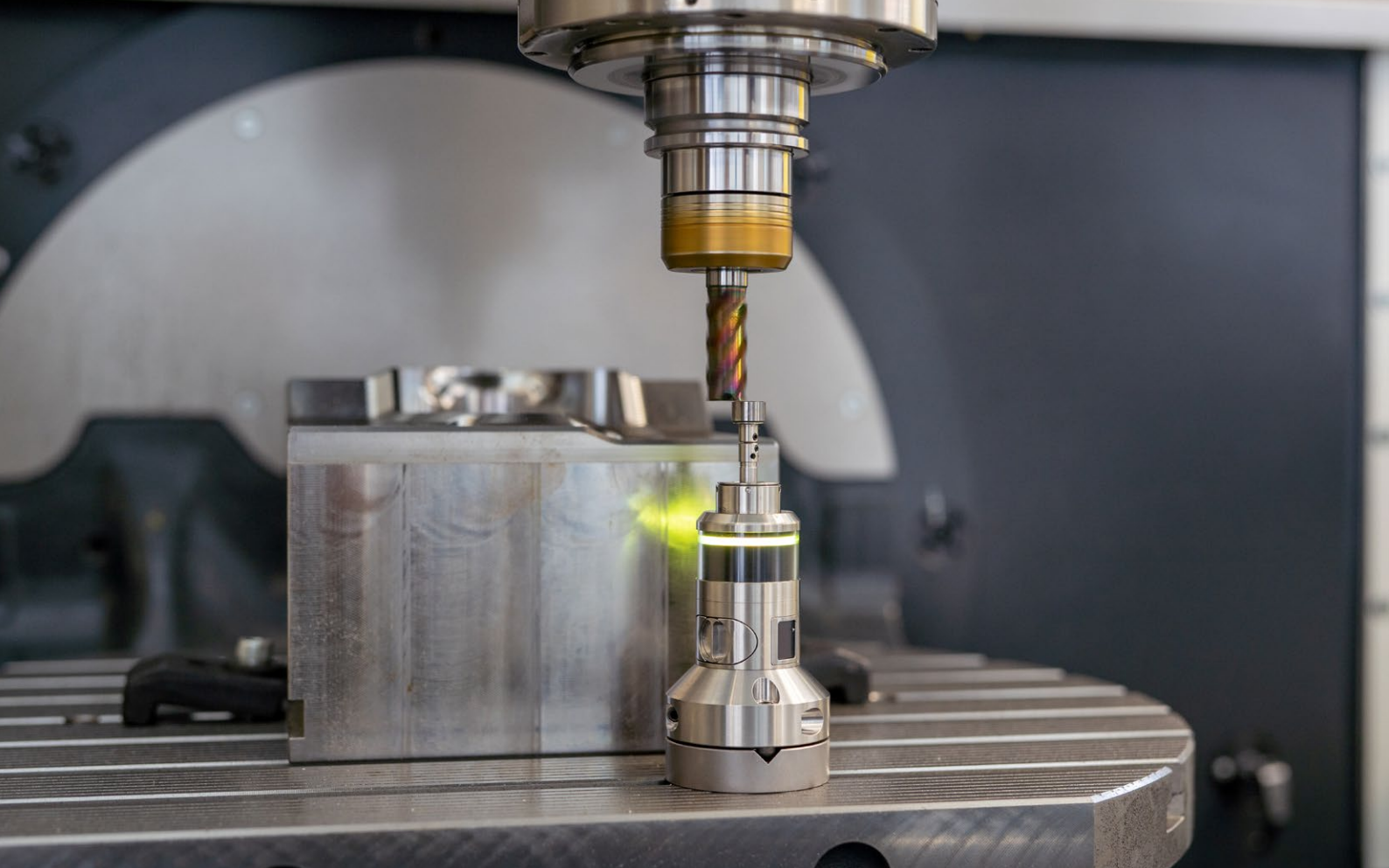
Figure 4. Touch probes are standard on almost every CNC production machine, and Hexagon's portfolio of probes with radio or infrared transmission benefit from many unique capabilities, such as the combination with other technologies, exchangeable measuring units and more.
