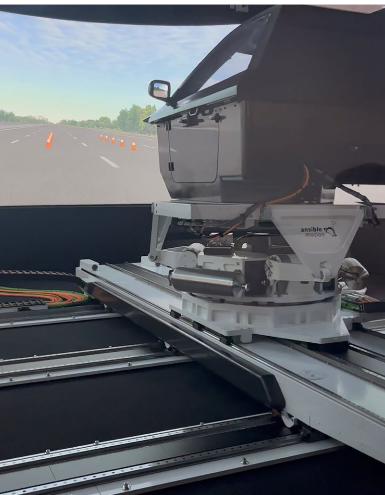
Figure1. Ansible Motion Dynamic Simulator Delta S3 with Adams Real Time and cosin FTire at NRDC.
