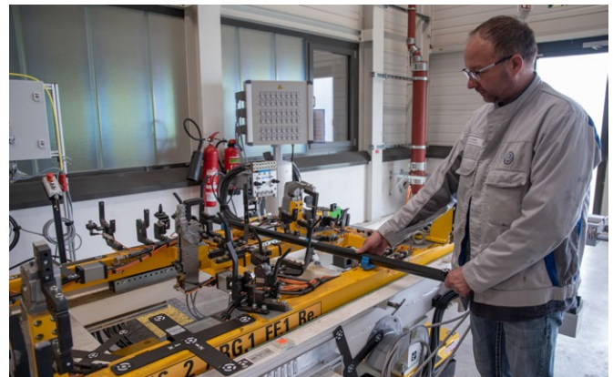
Figure 1. Before inspecting, the skid is signalled with scale bars, reference crosses and targets.
