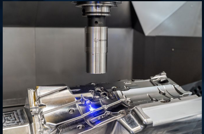
Figure 1. Laser scanners for machine tools can quickly capture the complete surface data for a part while it is still clamped, bringing new levels of speed, precision and flexibility to machine tool inspection.
