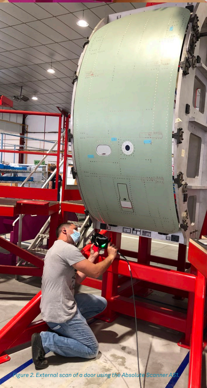
Figure 1. The Absolute Scanner AS1 quickly measures large and small parts.
