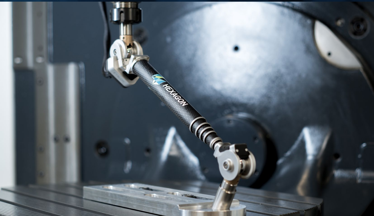
Figure 2. Automated wall thickness measurements on the machine tool with ultrasonic probes replace time-consuming manual measurements with external devices, without the need to move heavy and large parts to dedicated measurement spaces, ultimately resulting in significantly faster inspections and enhanced data capture.
