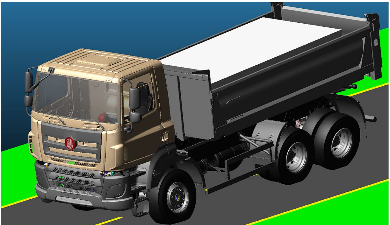
Figure 1. Braking simulations are used to validate that trucks will meet requirements and homologation for empty and loaded vehicles.
