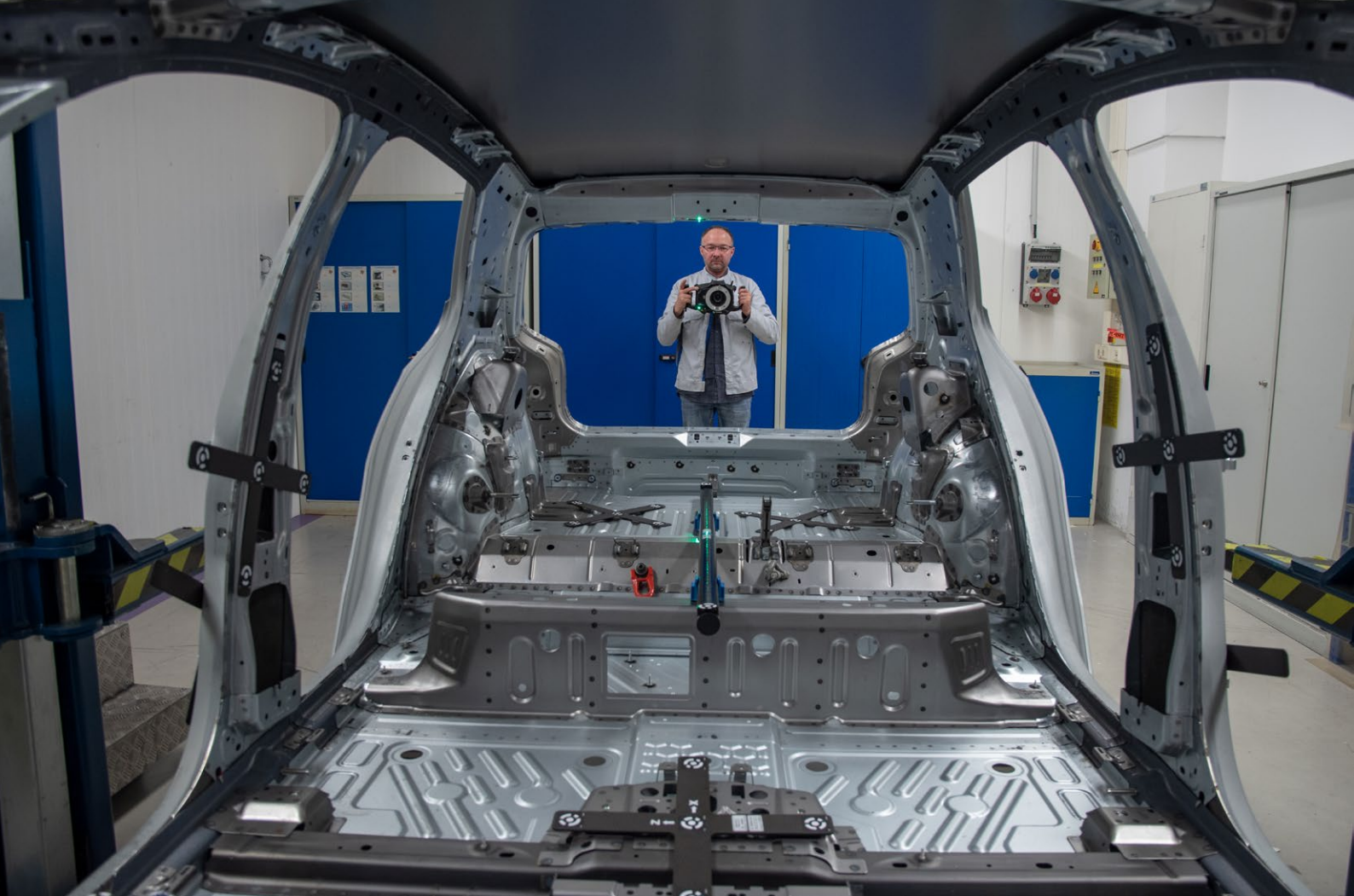
Figure 4. The point cloud created with the DPA Industrial is used to reference the handheld scanner.
