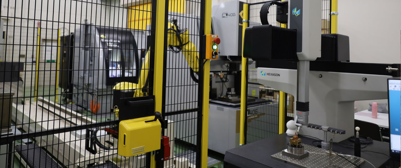
Figure 2. Hexagon's TIGO SF shop-floor CMM shown here in the Sodick Smart SITE semi-automated solution with the Sodick high-speed milling machine UH430L (rear left) and the Sodick die-sinker EDM machine AL40G (middle).
